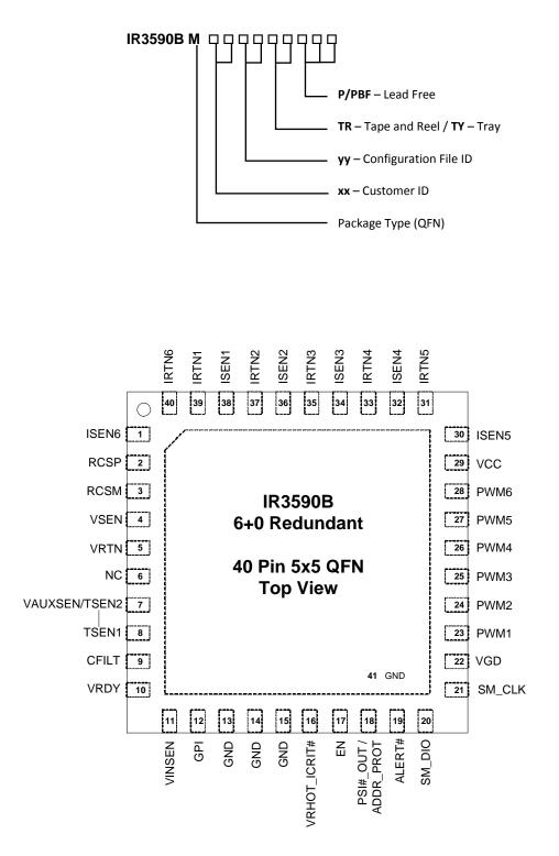
Figure 1: IR3590B Package Top View
