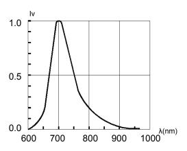
Fig. 1 Relative Luminous Intensity vs. Wavelength
