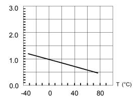
Fig. 3 Relative Luminous Intensity vs. Temperature
